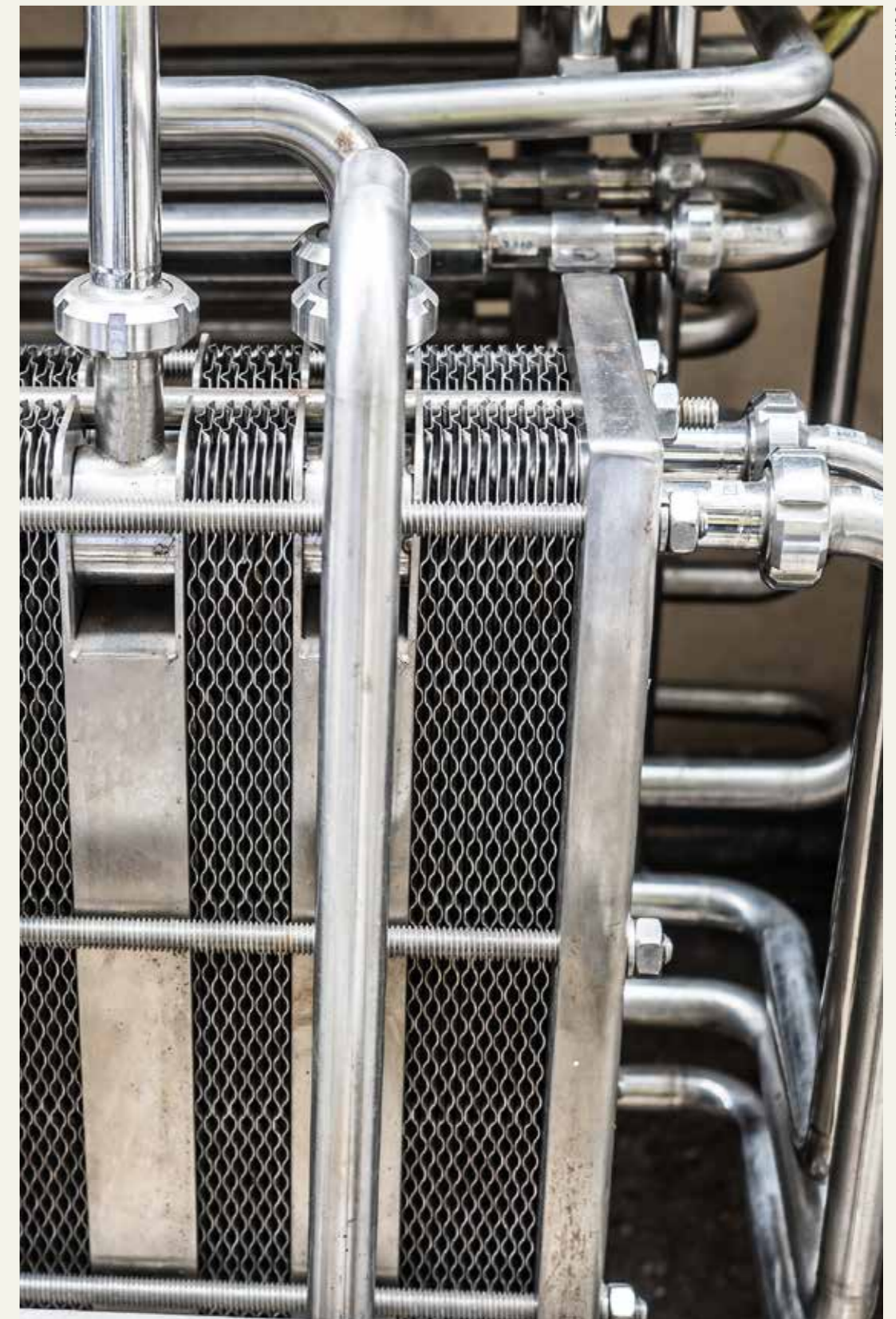
In solar water-heating systems, the heated medium is used to preheat the medium feeding into the collector using a heat exchanger. The heat is then stored in a well-insulated storage container.
